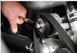
Use either a 15mm end wrench or ratchet and socket to release the tensioner assembly.
