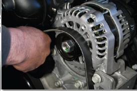
Take OEM Belt off of the alternator and remove from the engine compartment.
