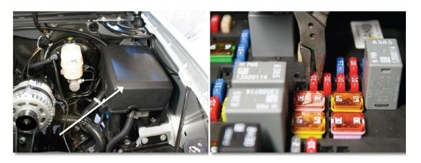
STEP 16: Install 10-amp fuse into provided fuse tap and re-install.
