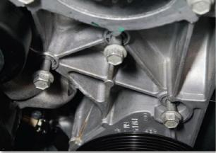
STEP 5: Loosen factory alternator mounting bolts and remove right hand bolt.
