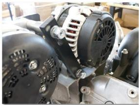
Attach Rear Support Bracket to the right hand rear of the factory alternator mounting bracket.
