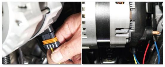
Attach the Red wire to the output post of the alternator. (Note: If blue wire is provided, attach along with red wire to output post.)
